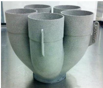
Figure 21 Collector made in alloy 625 with PBF- EB by Sandvik
