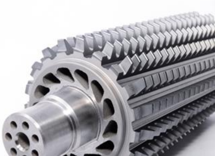
Figure 2 Milling cutter for gear manufacturing. The cutter is produced using AM in the material Vibenite®280, high alloyed HSS steel with an iron base, with a large number of carbides evenly distributed in the metallic matrix. Courtesy: VBN Components
