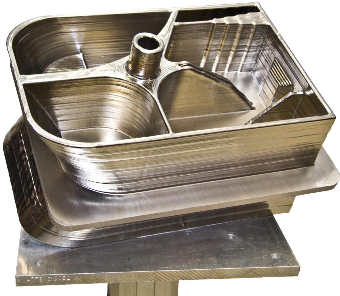
A box in Titanium, deposited by Laser Metal Deposition with wire. Picture courtesy of GKN Aerospace Engine Systems
